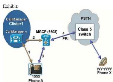
Assume that the gateway is a 6608 blade configured as a gateway and running MGCP; Call Manager runs version 3.1, and that a call is made from phone A to phone X. All IP streaming is G.711. Each of the logical links represented carries certain types of traffic. On which links can RTP traffic be seen?
